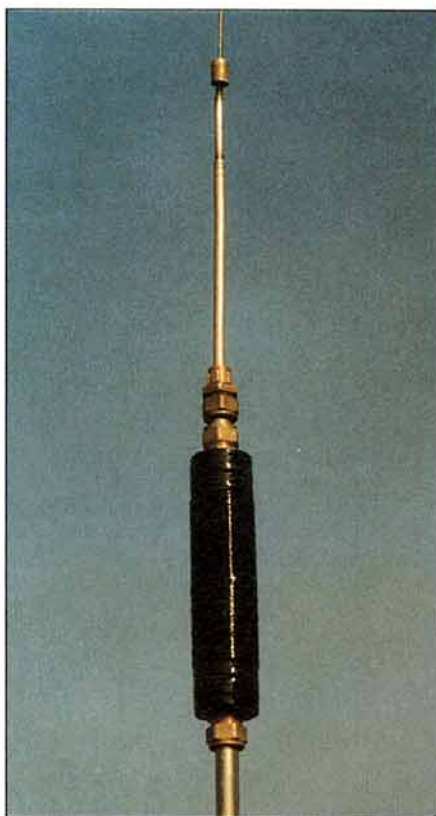
Fig 3: Coil former construction and dimensions will depend on the frequency in use.
